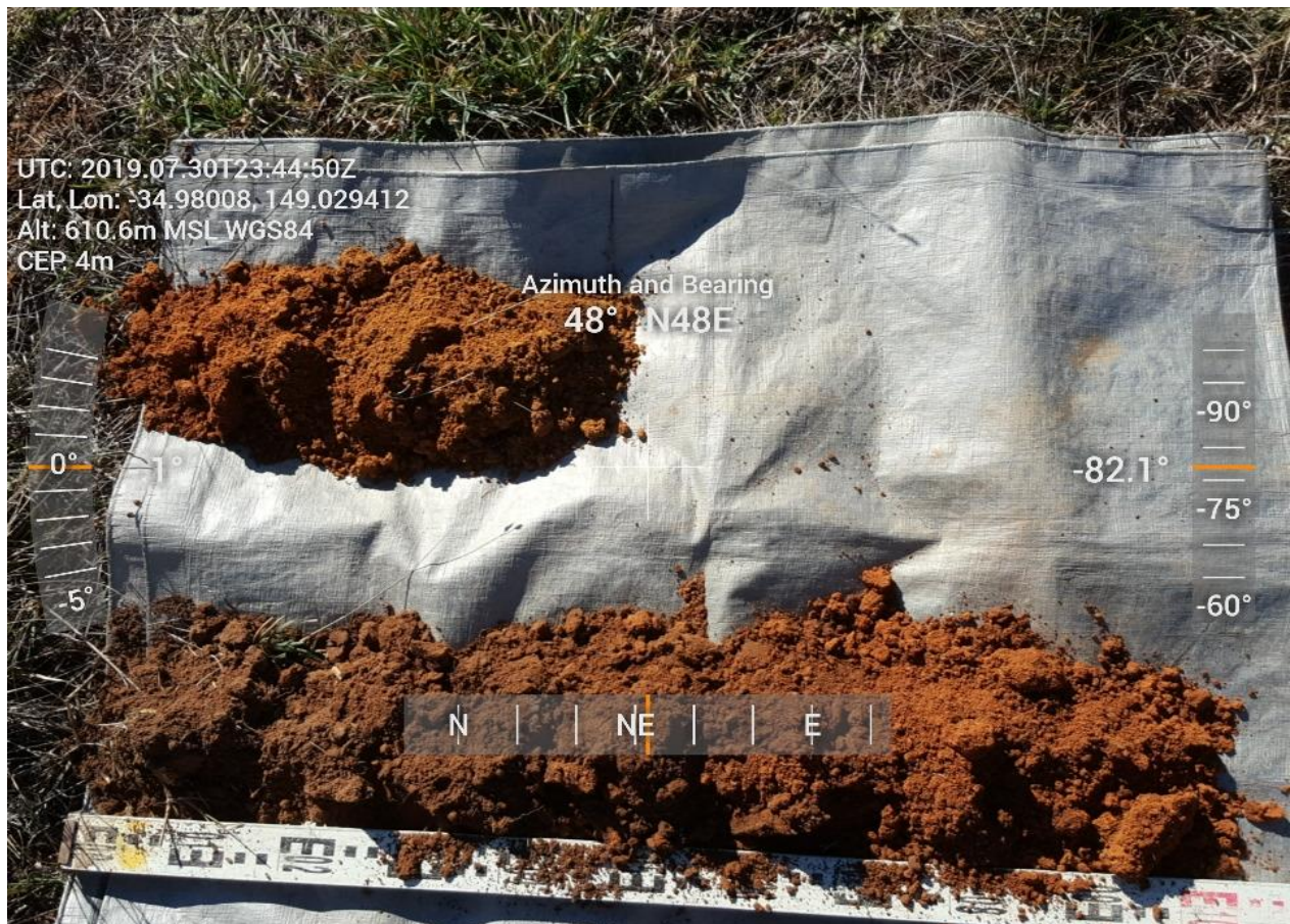
Figure 9: Lot 1 Building Envelope Soil Profile.
